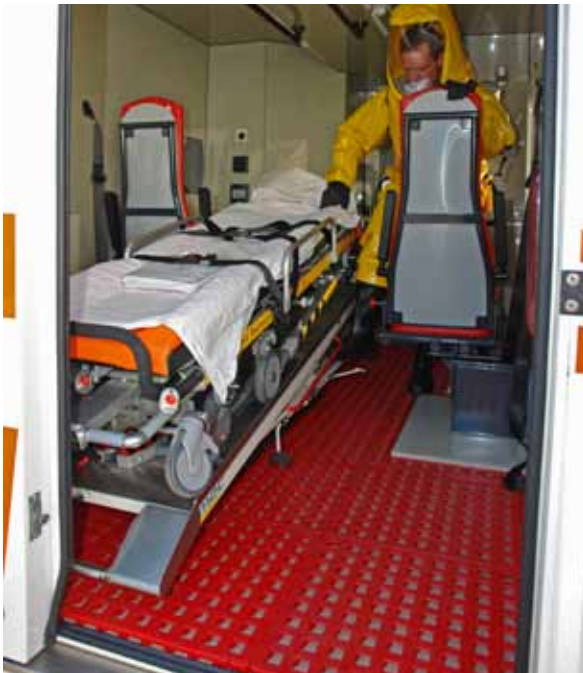
Dortmund Fire Brigade's ambulance for transporting patients with infectious diseases (source: Dortmund Fire Brigade)
