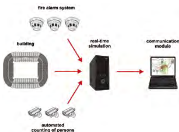
Principle diagram of the evacuation assistant (source: Hermes)
