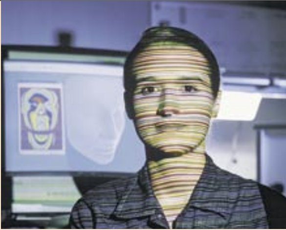
3D facial recognition: 3D object recognition using colour strips offers many fields of application.
